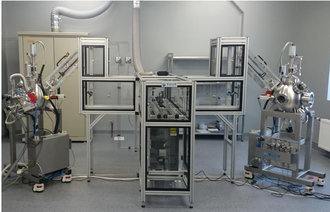
Two chamber PLD system – oxides and sulphides (900C max, 6 targets in a carousel)
